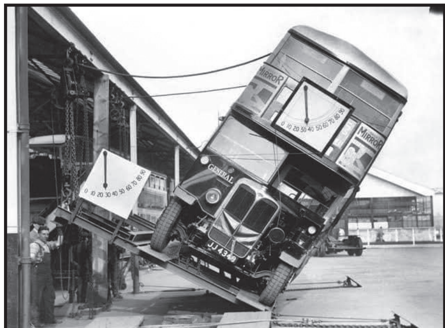
Bus "Center of Gravity" Test circa 1930
