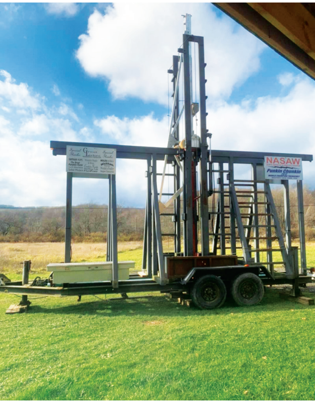
The trebuchet is a French style of catapult that has a counter weight and a sling that will add distance to a thrown object. They will begin launching pumpkins on the catapult at noon and will toss every half hour until dark.
